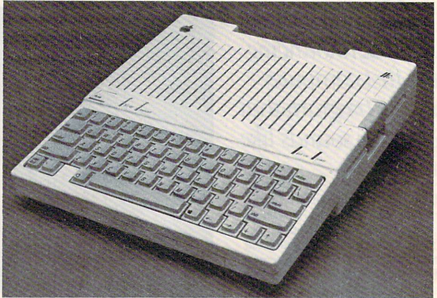
The $1295 Apple IIc, with a half-height 5¼-inch built-in disk drive on the right side, 128K RAM, and a 63-key keyboard, is a smaller, enhanced Apple IIe. (All photos courtesy of Apple Computer, Inc.)
